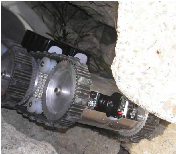
Fig. 10. RAPOSA moving out from a pipe within rubble.
