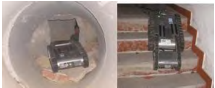
Fig. 2. The robot RAPOSA inside a sewer pipe and downstairs.
